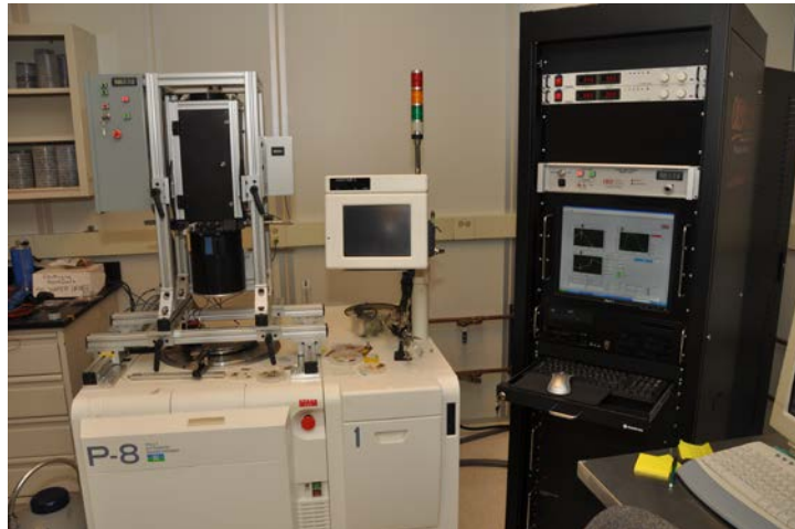
Figure 2: Photograph of Alpha-Omega flash tester employed to test ELO cells under concentration.
