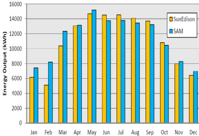
Fig. 1: Initial Comparison between SAM and Measured Data for the NREL S&TF Building
