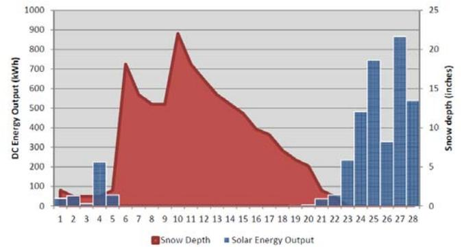
Fig. 2: Snow depth (red) and DC energy output (blue) for each day in February 2010, clearly showing the two Mid-Atlantic blizzards (6th and 10th) and the impact on solar energy generation.
