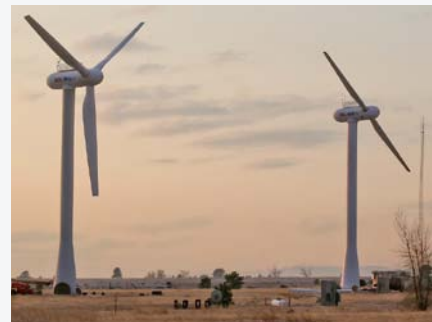
The three-bladed Controls Advanced Research Turbine (CART3) and the two-bladed CART2 are used to test new control schemes and equipment for reducing loads on wind turbine components. Photo by Lee Jay Fingersh, NREL/PIX 19937
