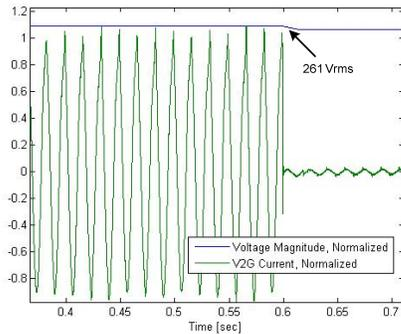
Fig. 3: Magnitude test for over voltage
