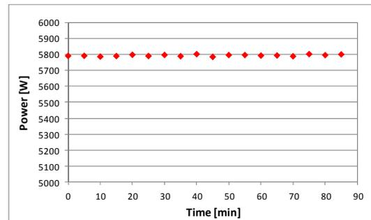
Fig. 9: V2G continuous output power
