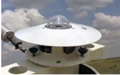
Fig. 1. Photograph of thermopile pyranometer. Source: NREL
