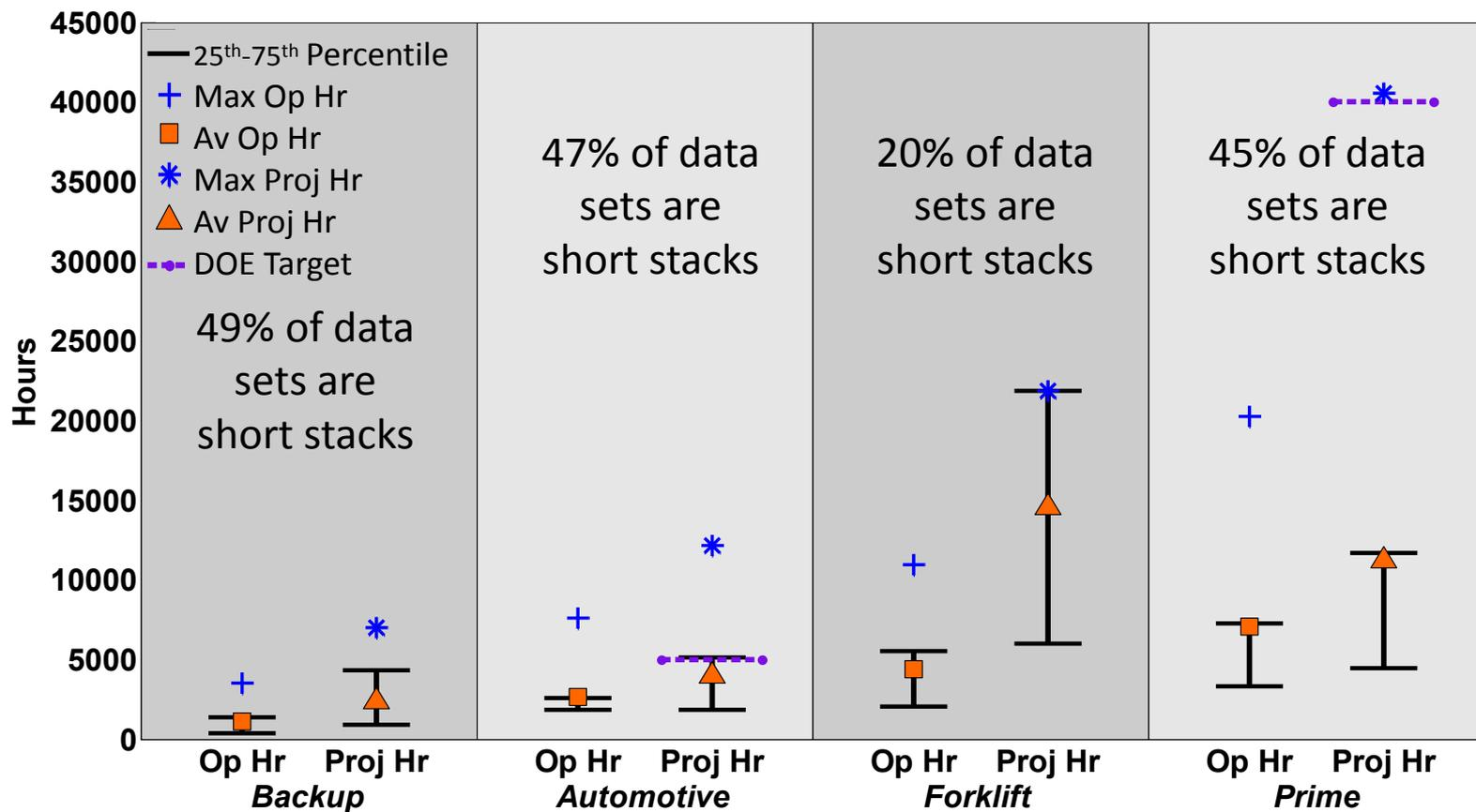
PEM & SOFC data from **lab tested**, full active area short stacks and systems with full stacks. Data generated from constant load, transient load, and accelerated testing and includes 10 fuel cell developers.
