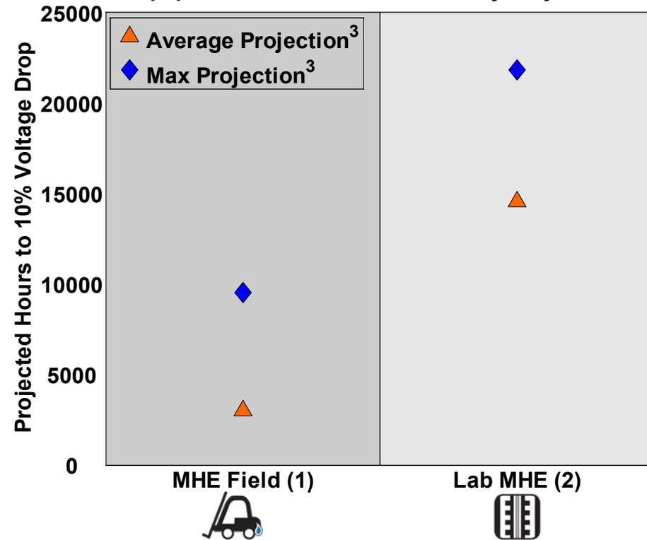
Comparisons in the automotive and material handling applications indicate there are **gaps between field and lab voltage durability performance**. Possible reasons include different data providers, technology generations, operating conditions, and test procedures. Additional comparisons to investigate are projections by configuration and test condition with field performance.
