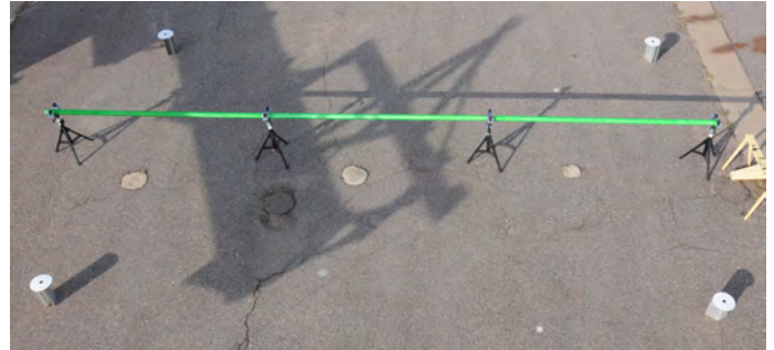
FIGURE 13. ABSORBER ALIGNMENT MEASUREMENT TEST SETUP WITH FOUR TARGETS AND MOCK ABSORBER
