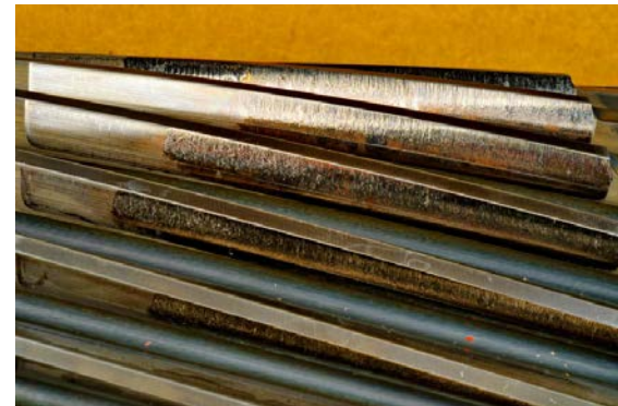
High-Speed Stage Pinion (Severe Scuffing) Photo from GEARTECH, NREL/PIX 19743
