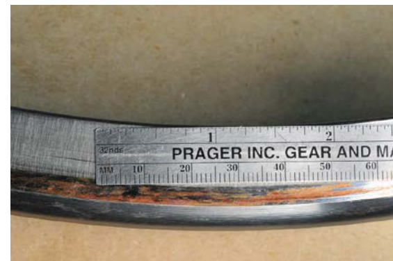
Bearing PLC-A Outer Raceway (Severe Fretting Corrosion) Photo from GEARTECH, NREL/PIX 19748
