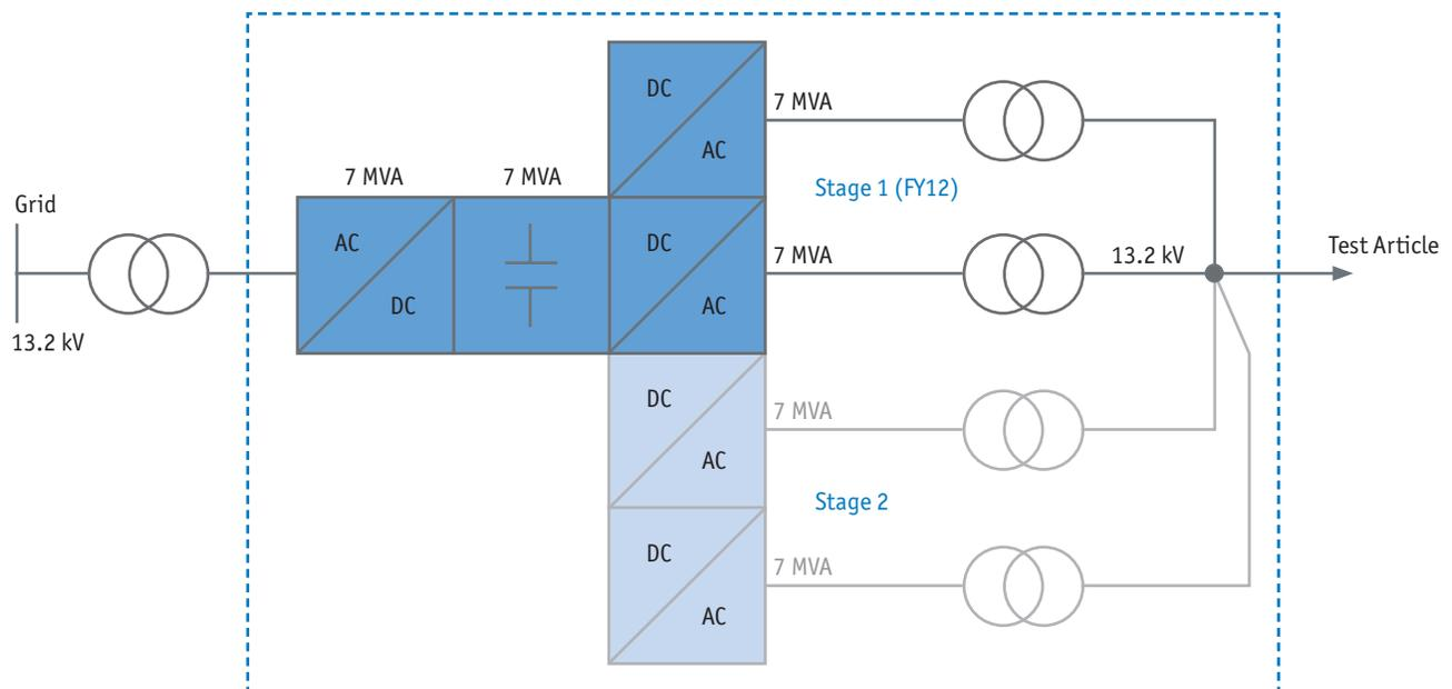
The electrical topology of the 7-MVA CGI consists of multiple voltage source converters. The line side converter is connected to the utility's 13.2 kV line, and two test article side converters are connected in parallel for increased short circuit current capability (14 MVA for stage 1). Up to 28 MVA short circuit current capability is possible with two additional parallel converters that will be added later if necessary. *Illustration by Vahan Gevorgian, NREL*
