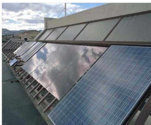
Fig. 1: Performance and Energy Ratings Testbed (PERT) at NREL. Photo credit: Warren Gretz, NREL PIX 03877.
