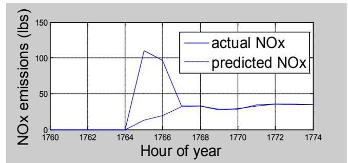
Fig. 8. Example of startup NO<sub>x</sub> emissions. Actual NO<sub>x</sub> measurements are shown by the solid blue line, and predicted NO<sub>x</sub> from the local linear fit is shown by the dashed blue line. Startup NO<sub>x</sub> emissions are defined as the difference between the actual NO<sub>x</sub> and predicted NO<sub>x</sub>.
