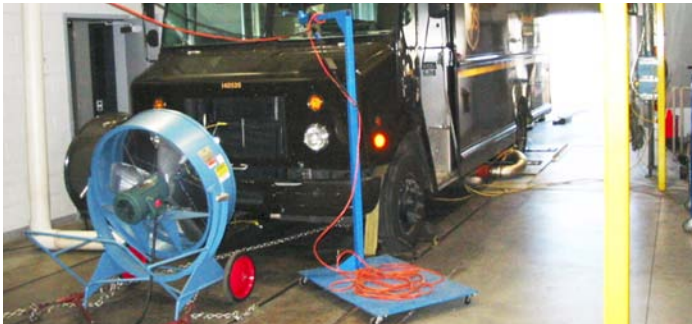
Parcel delivery vehicle on dynamometer. Photo by Jon Cosgrove, NREL/PIX 19813
