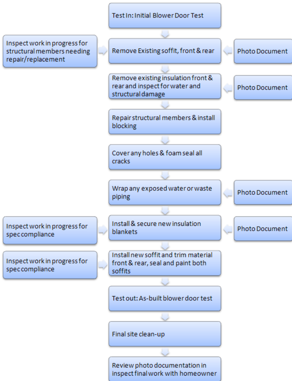
Figure 6. Construction process flow chart for a sealed and insulated cantilevered floor area
