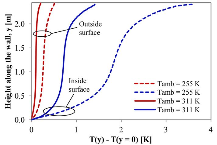
**Figure 4** Temperature profile along the vertical symmetry line of the internal and external surfaces of the wall. The graph shows changes in temperature relative to the bottom of the wall with an emissivity,  $\epsilon$ , of 0.8.
