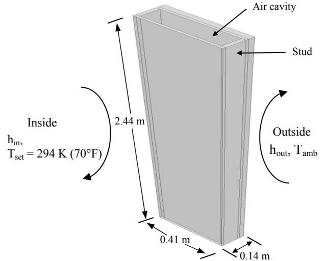
**Figure 1** Schematic of the wall structure, which consists of a  $0.41\text{-m}$  (16-in.) long  $\times$   $0.14\text{-m}$  (5.5-in.) wide  $\times$   $2.44\text{-m}$  (8-ft) high section of a standard  $2 \times 4$  residential stud wall.
