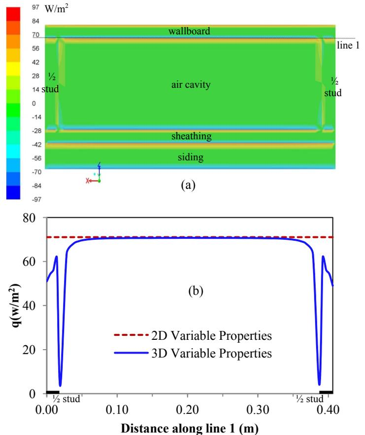
**Figure 8** Heat flux at ambient temperature of 233 K (-40°F) and emissivity of 0.8. (a) Distribution on the horizontal symmetry plane of the wall. (b) Profile on line 1 from right to left.
