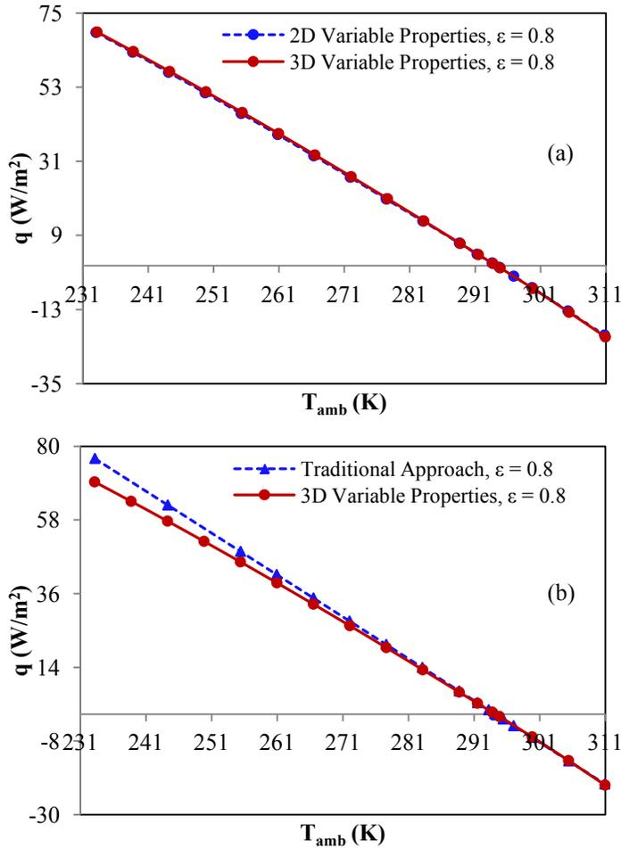
**Figure 9** Total heat flux through the wall assembly as a function of  $T_{amb}$  when the surface emissivity is 0.8. (a) comparison of 3D with 2D and (b) comparison of 3D with the traditional approach, assuming constant resistance evaluated at 297 K ( $75^\circ\text{F}$ ) mean temperature.
