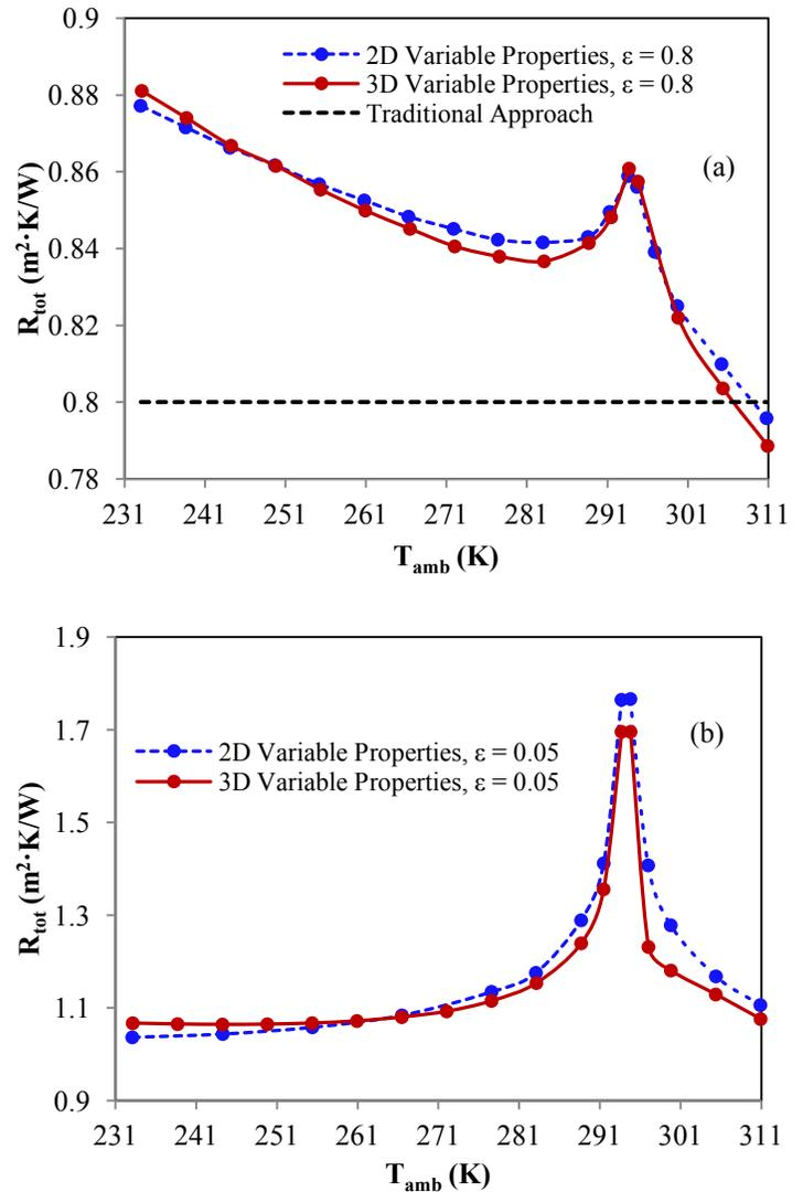
**Figure 6** Thermal resistance of the wall assembly, predicted using 2D and 3D models, as a function of the outdoor ambient temperature. (a) High surface emissivity of 0.8 and (b) low surface emissivity of 0.05.
