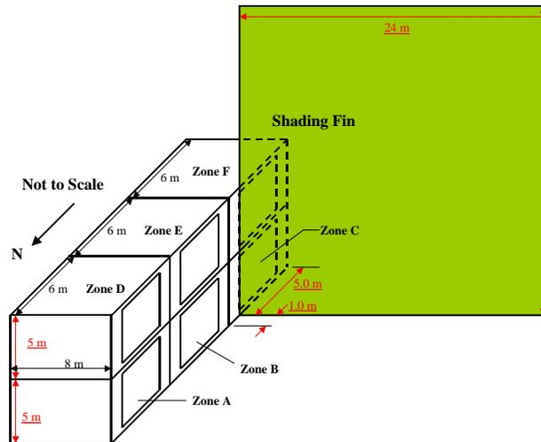
Figure 2 Multi-zone shading schematic (Neymark et al. 2008)
