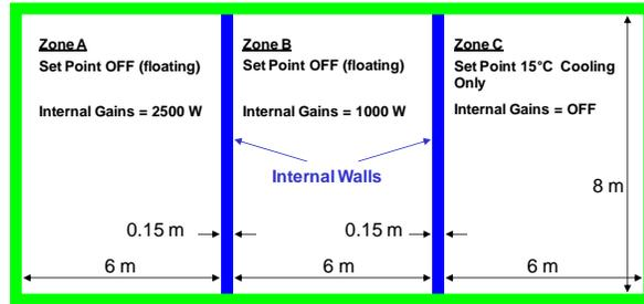
Figure 1 Multi-zone conduction schematic (Neymark et al. 2008)
