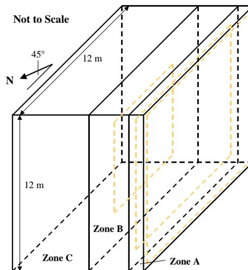
Figure 3 Multi-zone internal window schematic (Neymark et al. 2008)
