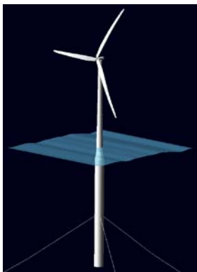
Figure 9: Illustration of NREL 5-MW wind turbine on OC3-Hywind spar (Jonkman et al., April 2010)
