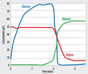
Glucose, xylose, and ethanol concentrations during enzymatic hydrolysis and fermentation of pretreated corn stover at 20% total solids. *Figure by NREL*
