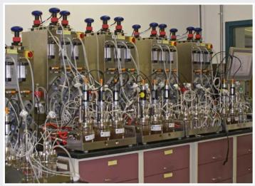
The 500-mL Biostat Q-Plus fermentors are used for small-scale fermentation testing. *Photo by Cindy Gerk, NREL/PIX 19431*
