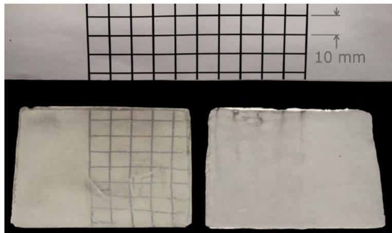
**Figure 1. Tin Direct Wafers. Left, surface on one side has mirror-like finish with excellent flatness, evidenced by reflection of grid. Right, Opposite surface is smooth, but not as flat. Credit: 1366 Technologies.**
