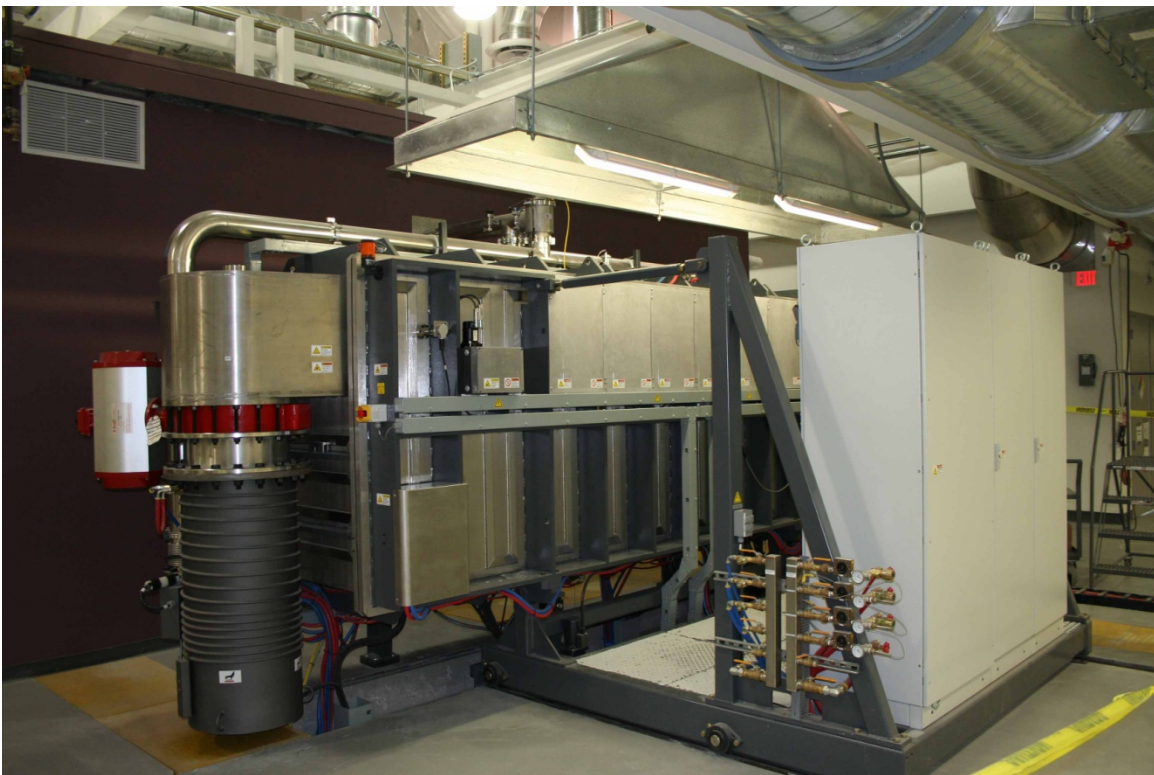
Fig. 2.7. A GSE tool for roll-to-roll absorber (CIGS) deposition at the new manufacturing facility in Tucson. (Credit: Global Solar Energy)
