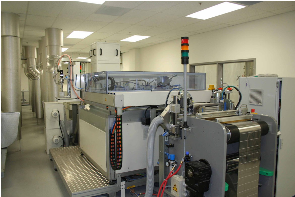
Fig. 2.8. Roll-to-Roll equipment for one of the “back-end” processes in the new factory (front contact collection grid printing). (Credit: Global Solar Energy)
