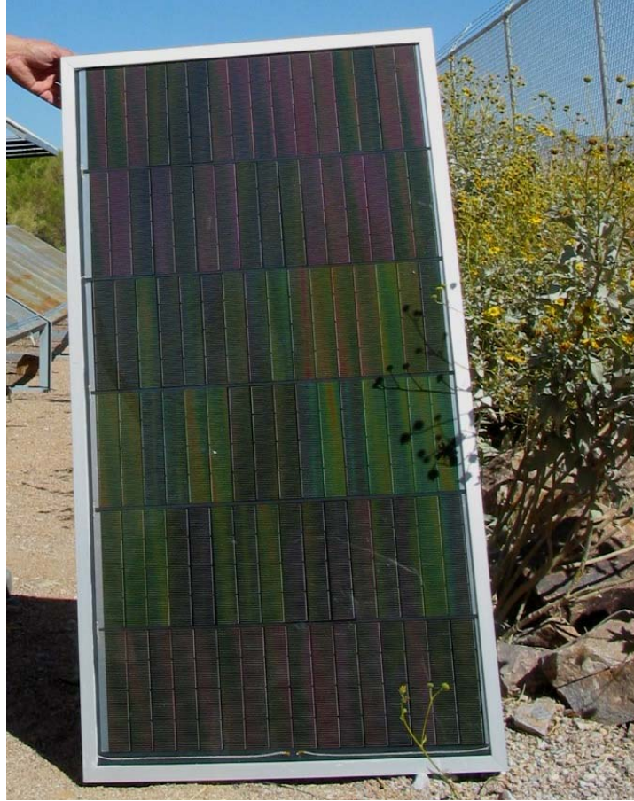
Fig. 1.13. An early large area product based on the Gen1 cell fabrication, and showing typical color variation due primarily to thickness variation in the initial CdS process. (Credit: Global Solar Energy)
