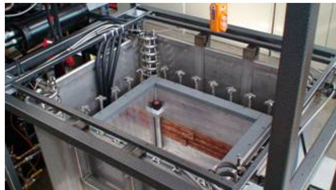
Calorimeter test chamber in isothermal fluid tank
