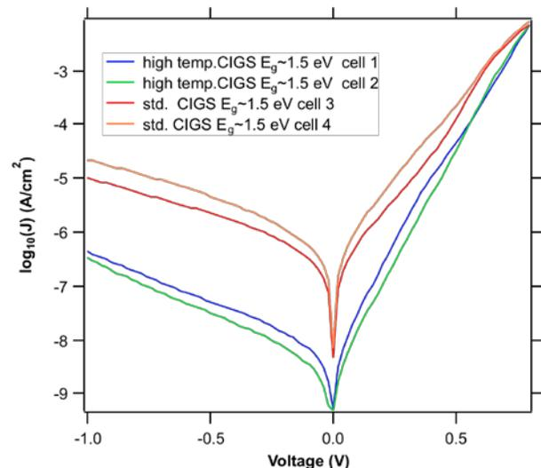
**Figure 4 Dark J-V curves for high temperature CIGS (lower curves) and standard CIGS (upper curves) solar cells with  $E_g \sim 1.5\text{ eV}$ .**
