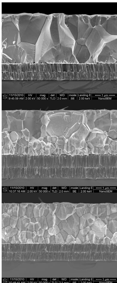
**Figure 5 Morphology of CIGS grown at 650 °C for  $x\sim 0.4$  (top),  $x\sim 0.5$  (middle) and  $x=1$  (bottom).**
