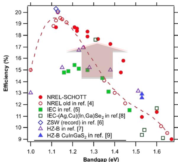
**Figure 1 Solar cell efficiency vs. CIGS absorber bandgap value.**
