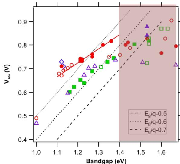
**Figure 2 V<sub>oc</sub> vs. CIGS absorber bandgap value. Data symbols as noted in Fig.1.**
