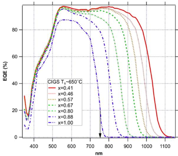
**Figure 3 External quantum efficiency curves for CIGS solar cells with absorbers grown at  $650^\circ\text{C}$ .**
