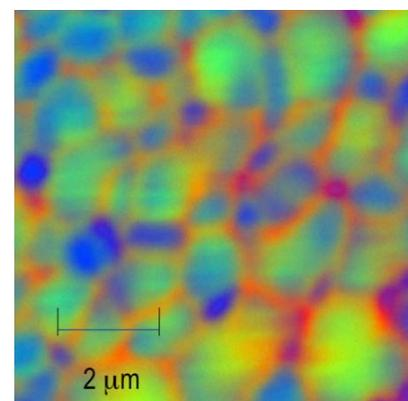
**Figure 9 Energy map of the CL emission from high temperature CIGS with  $x\sim 0.60$  (similar conditions as in Fig.8 were used).**
