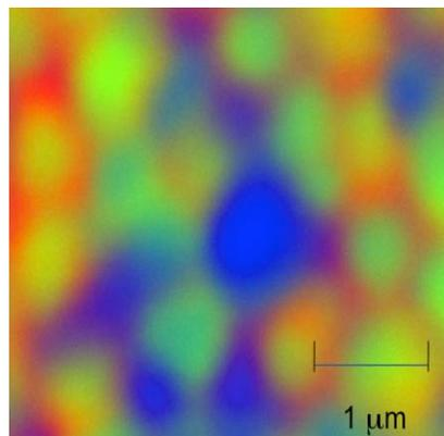
**Figure 8 Energy map map of the CL emission (at 1.260 eV, 80 meV energy window) from standard CIGS with  $x\sim 0.60$  from year 2003.**
