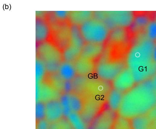
**Figure 7 Typical CL emission (a) linescan and (b) energy map at 1.130 eV, 80 meV energy window at grain interior (G1,G2) and at GB in high efficiency CIGS.**
