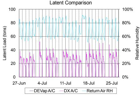
Figure 3-12 Latent load comparison and resultant space RH in Houston (DEVap A/C and DX A/C latent load profiles overlap)
