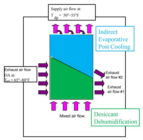
Figure 2-11 DEVap HMX air flows
