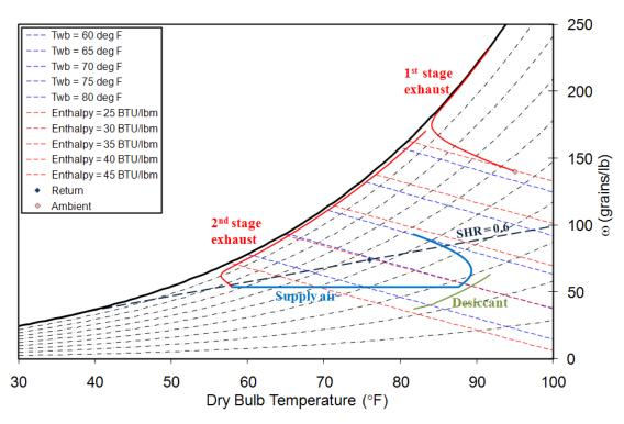
Figure 3-1 Temperature and humidity profiles of DEVap process using the Engineering Equation Solver model
