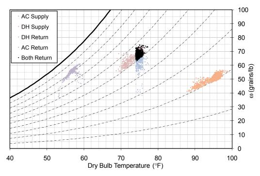
Figure 3-4 Return and supply air from the DX A/C and dehumidifier (shown as "DH") in a new residential building in Houston
