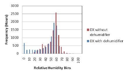
Figure 3-5 Effect of a whole-house dehumidifier when used with DX A/C in a new residential building in Houston
