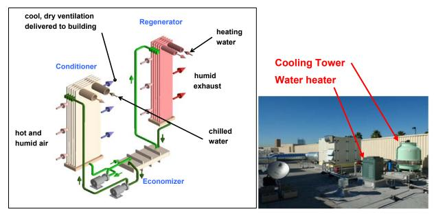
Figure 2-6 Major components and packaging of the AILR LDAC (Photograph shows packaged HMXs, water heater and cooling tower)
