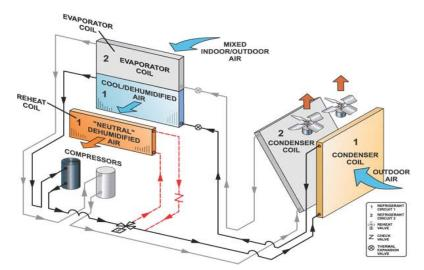
Figure 2-3 Lennox DX A/C with Humiditrol condenser reheat coil (Lennox Commercial 2010)
