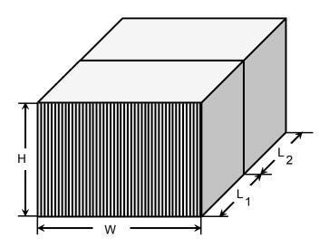
Figure 3-2 DEVap cooling core design
