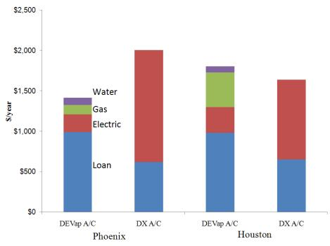
Figure 3-26 LCC breakdown for retrofit for Phoenix (hot, dry) and Houston (hot, humid) (loan is the repayment of the loan due to the upfront cost of each system)
