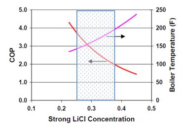
Figure 5-1 Vapor compression distillation regenerator latent COP using natural gas (AILR 2002) (shaded area shows operating range of the DEVap A/C)
