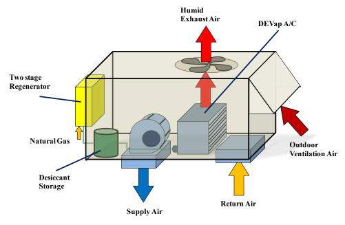
Figure 2-15 Example diagram of a packaged DEVap A/C
