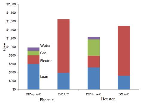
Figure 3-24 LCCs for residential new construction for Phoenix (hot, dry) and Houston (hot, humid) (loan is the repayment of the loan due to the upfront cost of each system)
