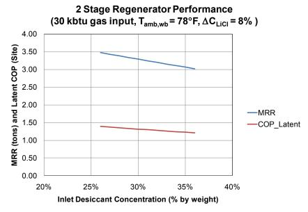
Figure 2-8 Calculated two-stage regenerator moisture removal rate and efficiency performance
