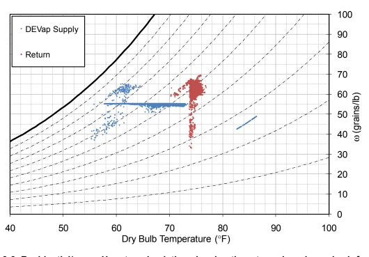
Figure 3-3 Residential/new – Houston simulation showing the return air and supply air from the DEVap A/C
