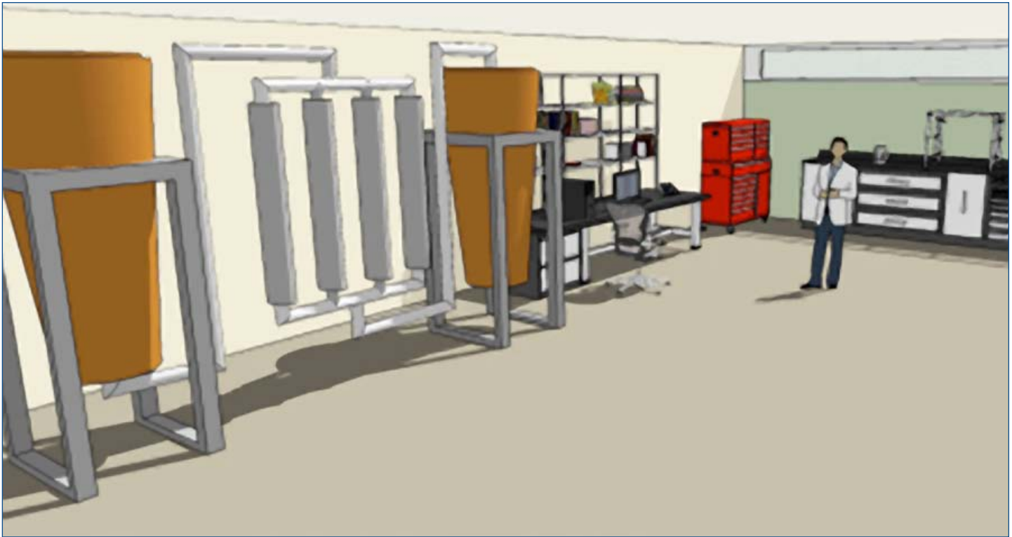
The Thermal Storage Process and Components Laboratory will operate in a temporary location while its permanent home, illustrated here, is developed on the NREL campus. Initial testing in the lab may relate to storing the thermal energy content of steam and will include the use of phase-change materials.
