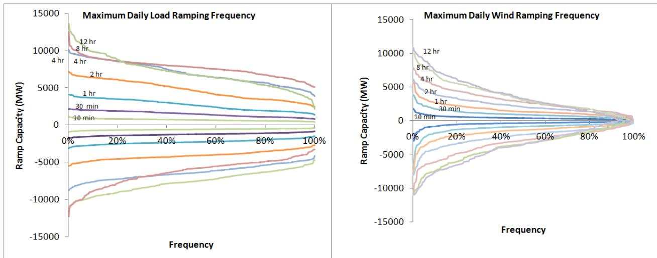
**Figure 6 – Maximum daily load and wind ramp frequency for ramps with durations from 10 mintes to 12 hours.**
