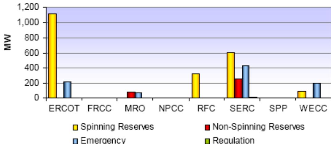
Figure 14 – Responsive loads are beginning to provide the fast ancillary services that are critical for reliability (NERC, 2009).
