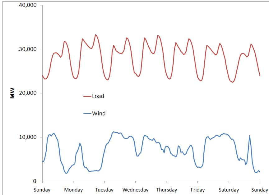
**Figure 2 – The slower, less predictable nature of wind is evident when compared with the typically daily load pattern.**
