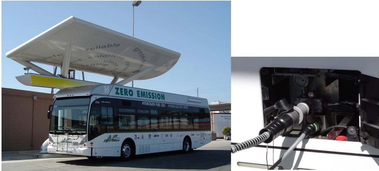
Figure 2. Fueling at the Chevron hydrogen station (Photo credit: L. Eudy, NREL)
