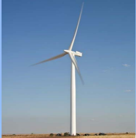
Figure 1. The Siemens SWT-2.3-101 prototype shown here at NREL's National Wind Technology Center illustrates current trends towards larger machines with larger rotors. These designs increase energy capture but questions remain regarding the cost effectiveness of continuing to scale turbines. PIX #17118.
