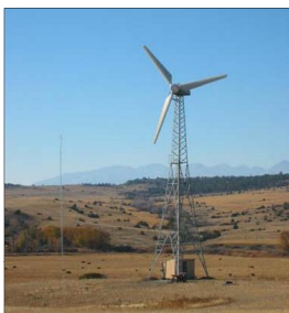
The 65 kW, refurbished Windmatic, erected by Tom Agnew at Agnew Farms. PIX #11947
