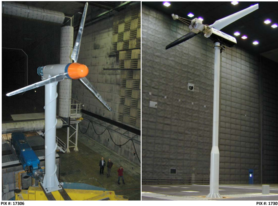
Figure 1. MEXICO turbine mounted in DNW 9.5 m x 9.5 m wind tunnel (left) and UAE Phase VI turbine mounted in NASA Ames 24.4 m x 36.6 m wind tunnel (right).
