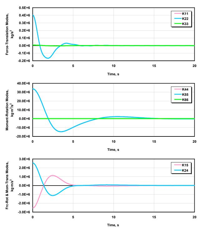
Figure 4-5. Radiation impulse-response functions for the OC3-Hywind spar
