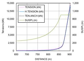
Figure 5-3. Load-displacement relationships for one OC3-Hywind mooring line
