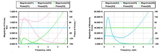
Figure 4-3. Hydrodynamic wave excitation per unit amplitude for the OC3-Hywind spar
