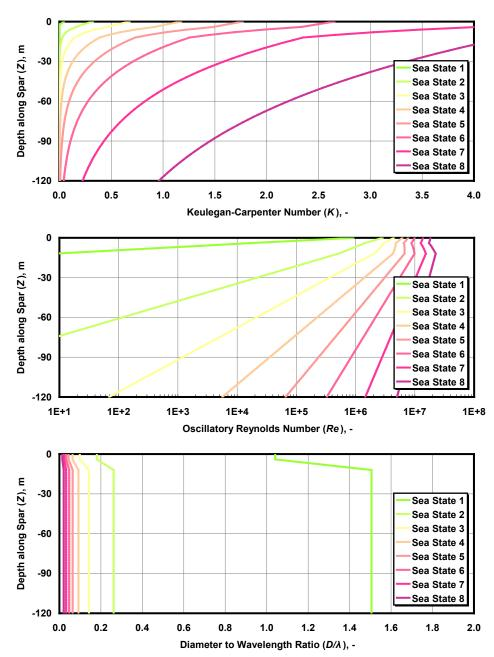
Figure 4-1. Dimensionless Parameters for the OC3-Hywind spar
