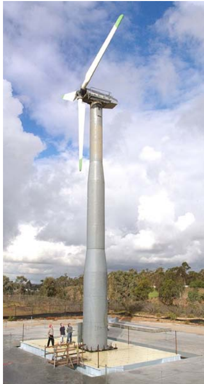
Figure 2. 65-kW Nordtank shake table test
