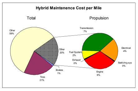
Figure 14. Propulsion maintenance cost per mile (hybrids)
