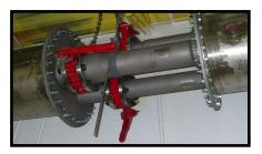
This allows the dilution level to be tailored to the engine size being tested (whether on the engine stand or in a
