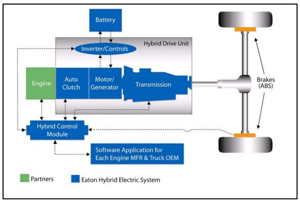
Figure 2. Eaton hybrid system schematic
