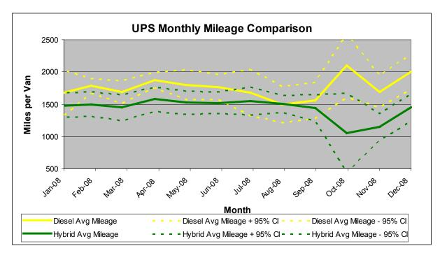
Figure 6. Hybrid and diesel monthly mileage per van
