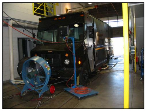
Figure 19. UPS P100 van on NREL's ReFUEL dynamometer
