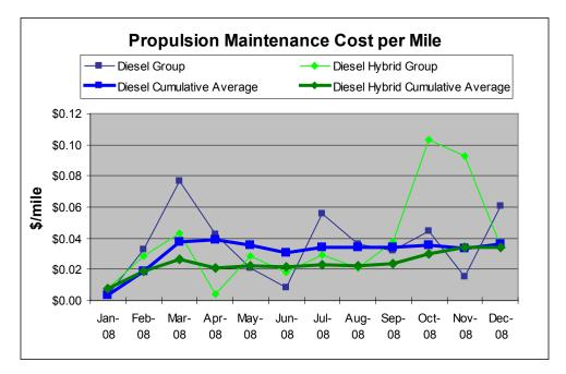
Figure 12. Propulsion maintenance cost per mile
