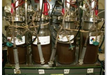
Bench scale conditioning, enzymatic hydrolysis and fermentation
