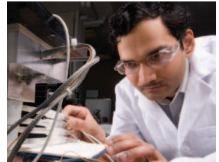
NREL's Sreekant Narumanchi watches the progress of temperature and pressure tests on materials used in hybrid automobile microelectronics.
