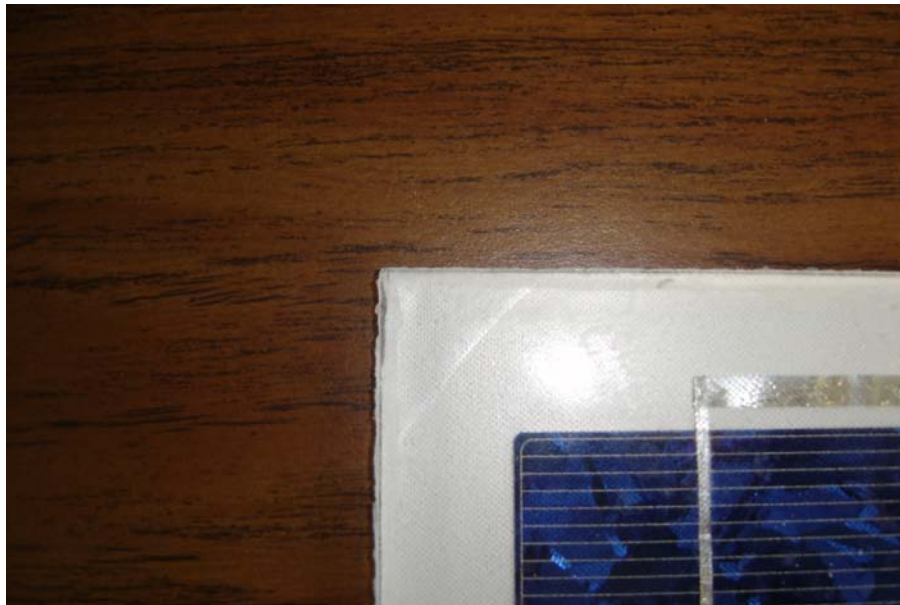
Figure 21 – Back Sheet Delamination after Thirty Three Humidity Freeze Cycles
