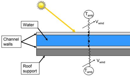
Fig. 2. Simple fully-wetted model for an unglazed collector.
