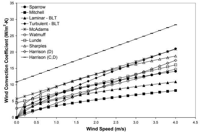
Fig. 4.  $h_{wind}$  vs.  $v_{wind}$  for 8 literature correlations, with  $L \sim .5$  m. The  $0.5$  m scale reduces the apparent discrepancies.
