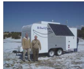
NREL's Mini-SODAR unit deployed at Fort Carson, CO site. Unit was installed alongside a 50-m Met tower. Mini-SODAR installed by Atmospheric Systems Corporation.
