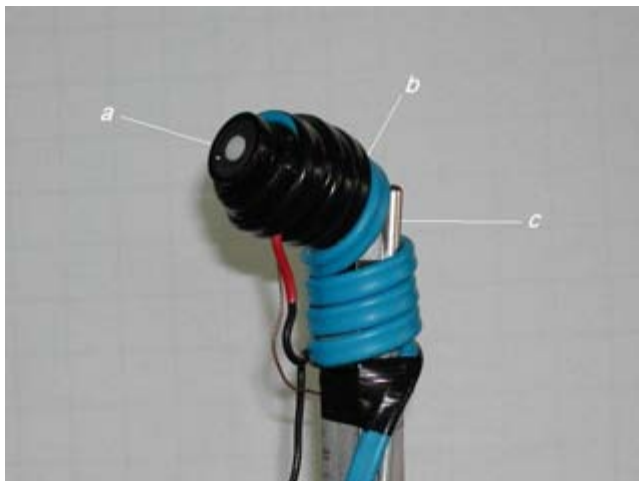
Fig. 1: Heated pyranometer components. (a) Li-Cor pyranometer, (b) heating cable, and (c) temperature sensor for temperature controller. The ends of the heating cable are secured with electrical tape.
