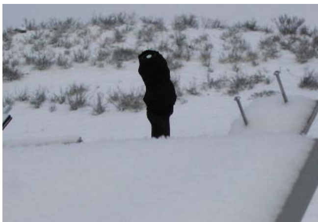
Fig. 2: Heated pyranometer demonstrating effectiveness in preventing snow and ice accumulation.
