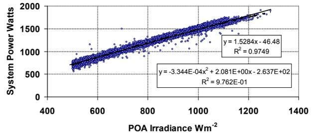
Fig 2. USSC Array data after filtering for non-standard operating conditions and for POA > 500 Wm<sup>-2</sup>
