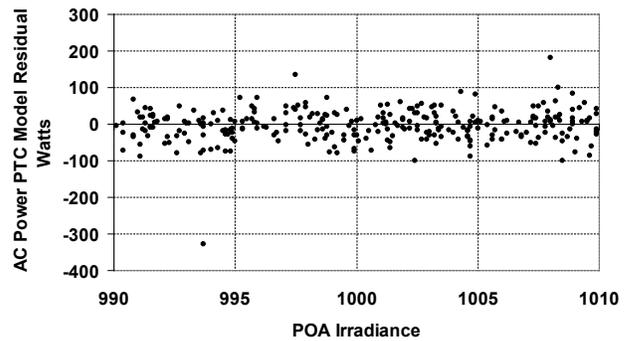
Fig. 3. Residuals (measured – modeled) of measured data from the PVUSA TC model line for irradiance levels from 990 Wm<sup>-2</sup> to 1000 Wm<sup>-2</sup>. Note this includes temperature range from -32.5 °C to 36 °C and wind speeds from 0.4 to 9.1 ms<sup>-1</sup>.
