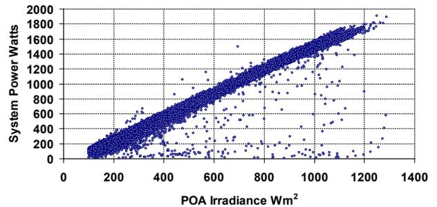
Fig 1. All raw USSC Array data versus plane of array irradiance for 2006
