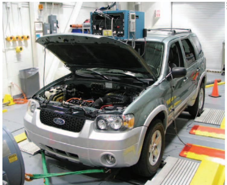
Chassis dynamometer emission testing
