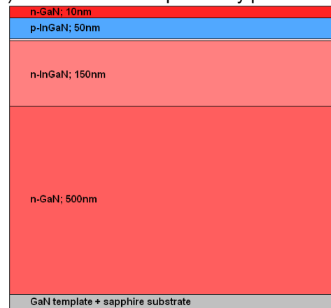
(c) Gen 3: Thickness of p-GaN reduced.
