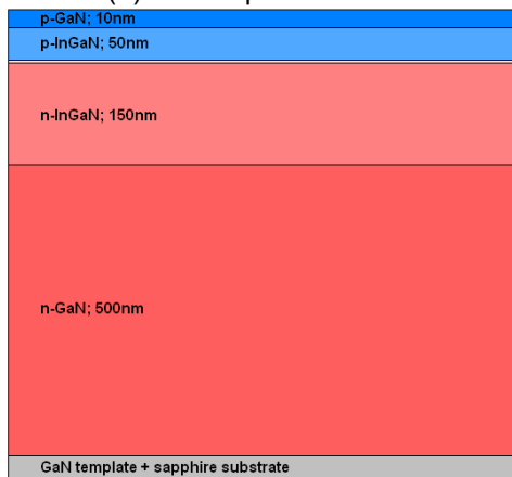
(c) Gen 3: Thickness of p-GaN reduced.
