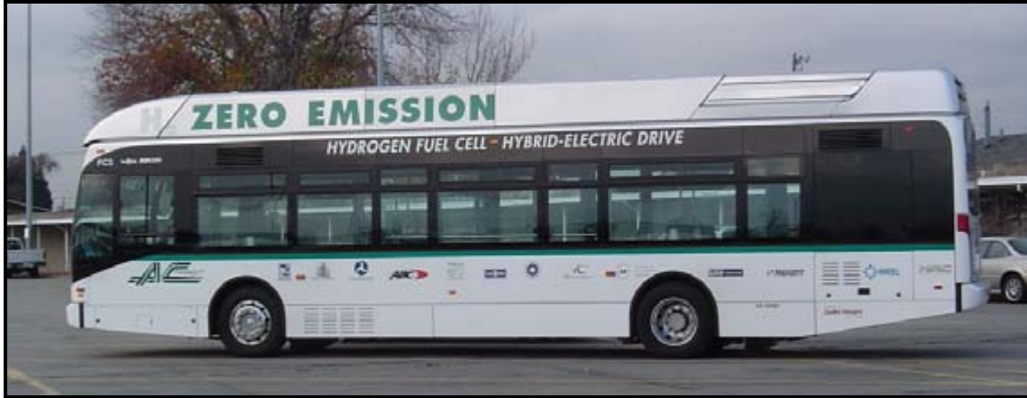
Figure B-1. AC Transit fuel cell bus
