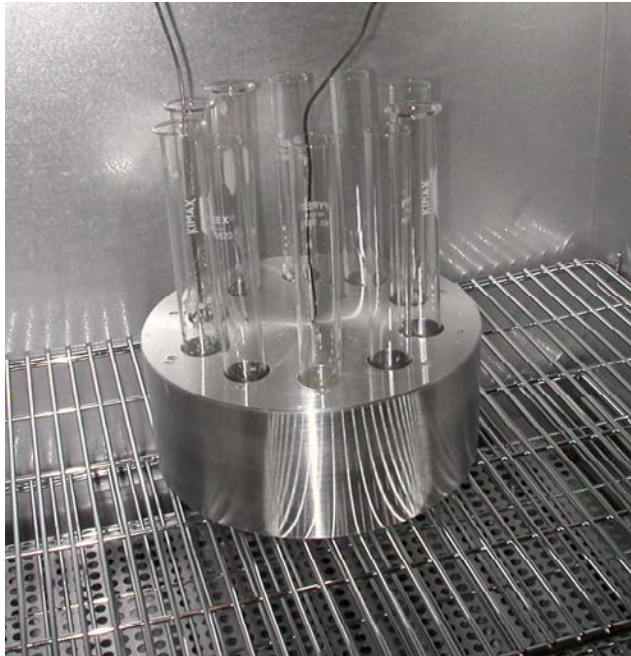
Mixture Composition vs. Solidification Testing Liquid Mixtures Observed at T < 100^\circ\text{C}
