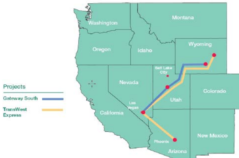
Figure 4. TransWest Express/Gateway South Transmission Projects
