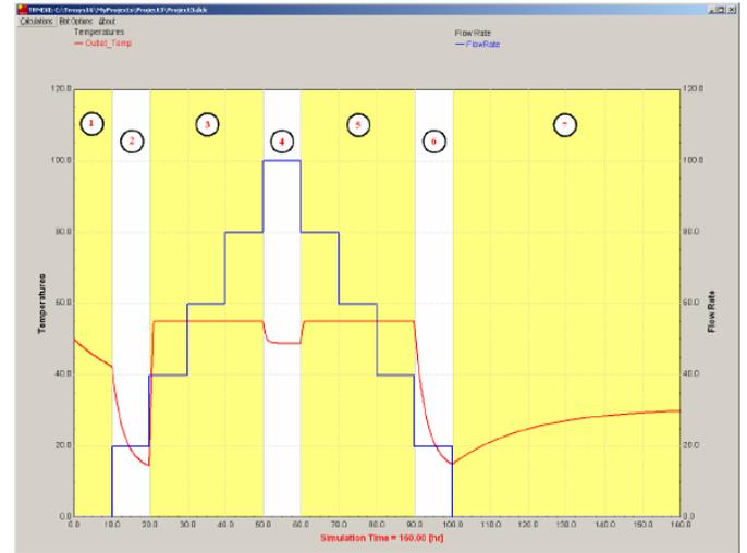
Fig. 4. Model response to varying flow rates. The red line is  $T_{out}$ , and the blue line is  $\dot{m}_{dot,in}$ .
