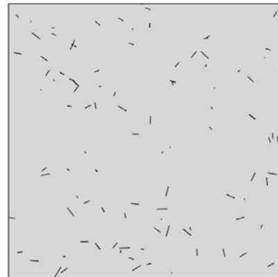
Fig. 2. Example of wafer with randomly distributed surface cracks used in Monte Carlo simulation. For legibility, the cracks are magnified 20 times.
