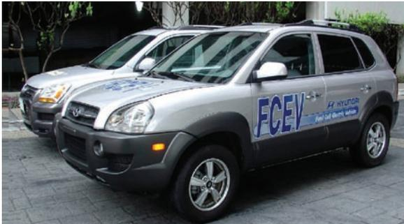
All of the teams are using polymer-electrolyte membrane fuel cells. Most of the vehicles have 350-bar (5,000-psi) compressed-hydrogen storage tanks, but a few have 700-bar (10,000-psi) or cryogenic liquid-hydrogen tanks. The fueling stations include a mixture of hydrogen delivered as a liquid and as compressed gas and on-site generation both by reformation of natural gas and by electrolysis.
