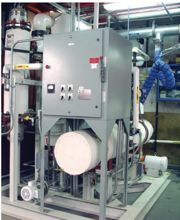
This evaporation system concentrates sugar-rich streams or removes volatile compounds.
