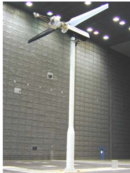
Figure 1. NREL Unsteady Aerodynamics Experiment wind turbine in NASA Ames 80 ft x 120 ft wind tunnel.
