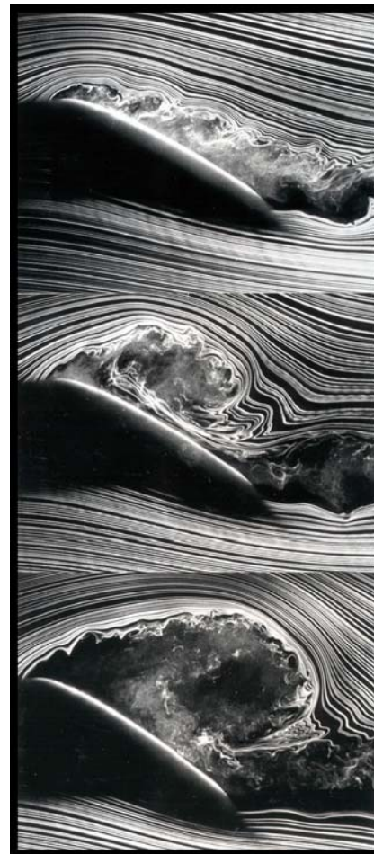
Figure 12. Smoke flow visualization of dynamic stall on an airfoil pitching in a wind tunnel.
