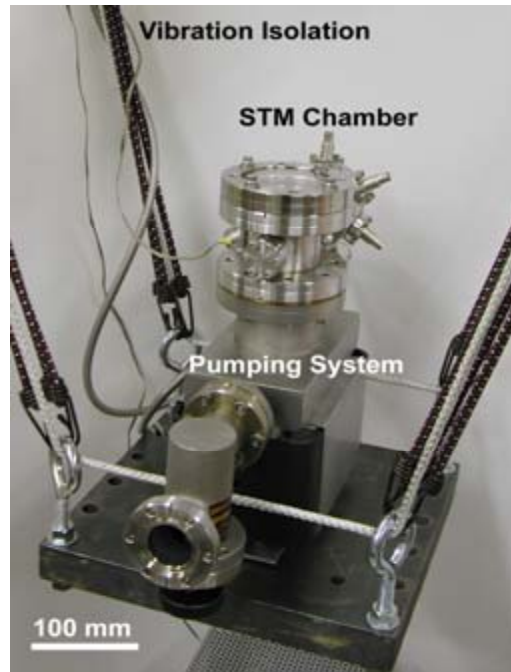
Figure 4.6 Compact UHV STM system for imaging and spectroscopy on solar cell materials.
