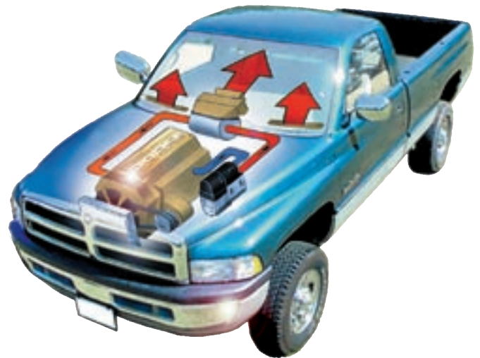
The auxiliary power unit draws low levels of energy from the truck’s engine to heat the cab without idling.
